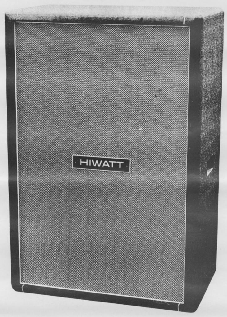
This enclosure is based on the popular reflex action which produces efficiencies 3-6dB louder over a conventional sealed system. Use is made of the effective rise in speaker impedance at low frequencies to match the port resistance in the range 50 to 150 c/s.
